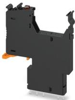
Safety plug adapter for use on a 6.2 mm PLC basic terminal block. For 5 x 20 mm fuses. Operating voltage: 120 ... 230 V AC/DC. With LED for fuse failure indication.
