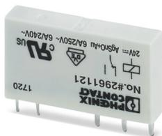
Plug-in miniature power relay, with multi-layer gold contact, 1 changeover contact, input voltage 24 V DC
