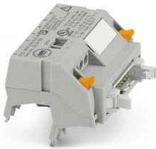
V8 adapter for 8 x PLC-INTERFACE (6.2 mm), controller: PLC system cabling of output cards, connection 1: IDC/FLK pin strip 1x 14-position, connection 2: Plug-in connection (Can be snapped onto 8x PLC-INTERFACE terminals), connection 3: Screw connection 1x 2-position, number of channels: 8, control logic: minusschaltend
