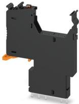
Safety plug adapter for use on a 6.2 mm PLC basic terminal block. For 5 x 20 mm fuses. Operating voltage: 12 ... 24 V AC/DC. With LED for fuse failure indication.
