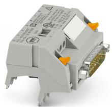
V8 adapter for 8 x PLC-INTERFACE (6.2 mm), controller: PLC system cabling of output cards, connection 1: D-SUB pin strip 1x 15-position, connection 2: Plug-in connection (Can be snapped onto 8x PLC-INTERFACE terminals), connection 3: Screw connection 1x 2-position, number of channels: 8, control logic: plusschaltend
