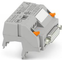
V8 adapter for 8 x PLC-INTERFACE (6.2 mm), controller: PLC system cabling of output cards, connection 1: D-SUB socket strip 1x 15-position, connection 2: Plug-in connection (Can be snapped onto 8x PLC-INTERFACE terminals), connection 3: Screw connection 1x 2-position, number of channels: 8, control logic: plusschaltend
