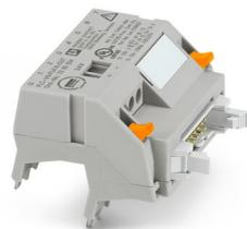
V8 adapter for 8 x PLC-INTERFACE (6.2 mm), controller: PLC system cabling of output cards, connection 1: IDC/FLK pin strip 1x 14-position, connection 2: Plug-in connection (Can be snapped onto 8x PLC-INTERFACE terminals), connection 3: Screw connection 1x 2-position, number of channels: 8, control logic: plusschaltend
