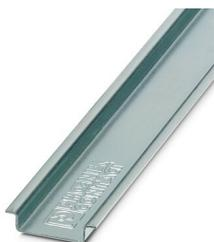
DIN rail, unperforated, acc. to EN 60715, material: Steel, Galvanized, white passivated, Standard profile, color: silver, Pack of 10 (20 m)
