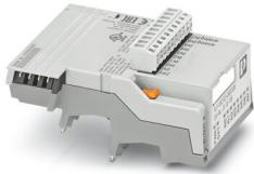
PLC logic extension module with 16 I/Os, for plug-in connection to eight PLC-INTERFACE terminal blocks for extending the basic module (a maximum of two extension modules can be connected to a basic module), screw connection
