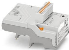
PLC logic basic module with RS-485 connection for Modbus/RTU communication, with 16 I/Os, for plug-in connection to 8 digital or analog PLC-INTERFACE terminal blocks, can be extended to 48 I/Os, real-time clock, micro USB female connector, accommodates memory module and Bluetooth adapter, Push-in connection
