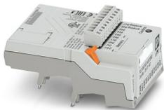
PLC logic basic module, Generation 2, with 16 I/Os, for plug-in connection to eight digital or analog PLC-INTERFACE terminal blocks, can be extended to 48 I/Os, real-time clock, micro USB female connector, accommodates memory module and Bluetooth adapter, screw connection
