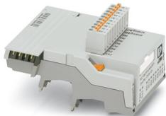
PLC logic extension module with 16 I/Os, for plug-in connection to eight PLC-INTERFACE terminal blocks for extending the basic module (a maximum of two extension modules can be connected to a basic module), Push-in connection
