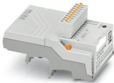
PLC logic stand-alone module, Generation 2, with 16 I/Os, for plug-in connection to eight digital or analog PLC-INTERFACE terminal blocks, cannot be extended, real-time clock, micro USB female connector, accommodates memory module and Bluetooth adapter, Push-in connection
