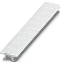
Marker for terminal blocks, Strip, white, labeled, can be labeled with: CMS-P1-PLOTTER, horizontal: L1, L2, L3, N, PE, L1, L2, L3, N, PE, mounting type: snapped, for terminal block width: 6.2 mm, lettering field size: 6.15 x 10.5 mm, Number of individual labels: 10
