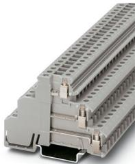
Sensor/actuator terminal block, nom. voltage: 250 V, nominal current: 24 A, connection method: Screw connection, 1st, 2nd and 3rd level, Rated cross section: 2.5 mm<sup>2</sup>, cross section: 0.2 mm<sup>2</sup> - 4 mm<sup>2</sup>, mounting type: NS 35/7,5, NS 35/15, color: gray
