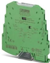
MCR 3-way isolation amplifier, with configurable input/output, for electrical isolation and conversion of analog signals up to 30 V, with screw connection, standard configuration
