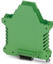
DIN rail housing, Lower housing part with metal foot catch, with FE contact, tall design, with vents, width: 22.6 mm, height: 99 mm, depth: 107.3 mm, color: green (6021), cross connection: integrated bus connector, number of positions cross connector: 10+2, Bus connector: 10 parallel contacts, 2 serial contacts
