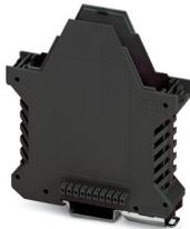
DIN rail housing, Lower housing part with metal foot catch, with FE contact, tall design, with vents, width: 22.6 mm, height: 99 mm, depth: 107.3 mm, color: black (9005), cross connection: integrated bus connector, number of positions cross connector: 10, Bus connector: 10 parallel contacts
