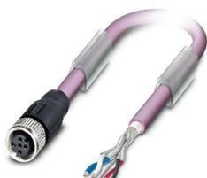
Bus system cable, CANopen<sup>®</sup>, DeviceNet<sup>™</sup>, 5-position halogen-free, shielded, free cable end, on Socket straight M12, coding: A, cable length: 5 m
