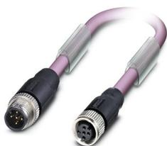
Bus system cable, CANopen<sup>®</sup>, DeviceNet<sup>™</sup>, 5-position halogen-free, shielded, Plug straight M12, coding: A, on Socket straight M12, coding: A, cable length: 2 m
