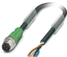
Sensor/actuator cable, 4-position, Plug straight M12, coding: A, connected with unwired, on free cable end, cable length: 10 m
