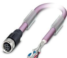
Bus system cable, CANopen<sup>®</sup>, DeviceNet<sup>™</sup>, 5-position halogen-free, shielded, free cable end, on Socket straight M12, coding: A, cable length: 2 m
