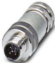
Data connector, CAN Bus/DeviceNet, 5-position, shielded, Plug straight M12, A, Screw connection, knurl material: Zinc die-cast, nickel-plated, cable gland Pg9, external cable diameter 6.5 mm ... 8.5 mm
