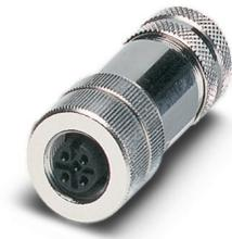
Data connector, CAN Bus/DeviceNet, 5-position, shielded, Socket straight M12, A, Screw connection, knurl material: Zinc die-cast, nickel-plated, cable gland Pg9, external cable diameter 6.5 mm ... 8.5 mm
