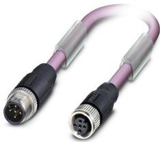
Bus system cable, CANopen<sup>®</sup>, DeviceNet<sup>™</sup>, 5-position halogen-free, shielded, Plug straight M12, coding: A, on Socket straight M12, coding: A, cable length: 15 m
