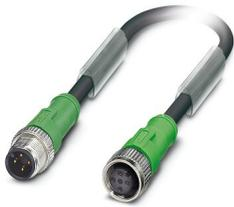
Sensor/actuator cable, 4-position, Plug straight M12, coding: A, connected with unwired, on Socket straight M12, coding: A, cable length: 2 m
