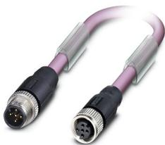
Bus system cable, CANopen<sup>®</sup>, DeviceNet<sup>™</sup>, 5-position halogen-free, shielded, Plug straight M12, coding: A, on Socket straight M12, coding: A, cable length: 0.5 m
