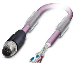
Bus system cable, CANopen<sup>®</sup>, DeviceNet<sup>™</sup>, 5-position halogen-free, shielded, Plug straight M12, coding: A, on free cable end, cable length: 15 m
