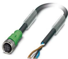
Sensor/actuator cable, 4-position, free cable end, on Socket straight M12, coding: A, cable length: 15 m
