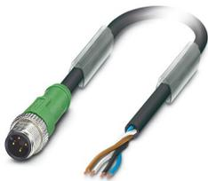
Sensor/actuator cable, 4-position, Plug straight M12, coding: A, connected with unwired, on free cable end, cable length: 2 m
