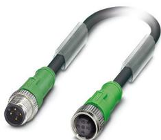
Sensor/actuator cable, 4-position, Plug straight M12, coding: A, connected with unwired, on Socket straight M12, coding: A, cable length: 0.5 m
