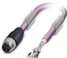
Bus system cable, CANopen<sup>®</sup>, DeviceNet<sup>™</sup>, 5-position halogen-free, shielded, Plug straight M12, coding: A, on free cable end, cable length: 10 m
