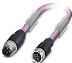
Bus system cable, CANopen<sup>®</sup>, DeviceNet<sup>™</sup>, 5-position halogen-free, shielded, Plug straight M12, coding: A, on Socket straight M12, coding: A, cable length: 1 m
