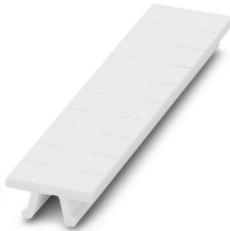
Zack marker strip, Strip, white, unlabeled, can be labeled with: PLOTMARK, CMS-P1-PLOTTER, mounting type: snapped, for terminal block width: 5.08 mm, lettering field size: 4.98 x 10.5 mm, Number of individual labels: 10
