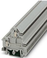
Double-level modular terminal block with COMBICON plug-in zone, nominal current: 12 A, nominal voltage: 250 V, cross section: 0.2 mm<sup>2</sup> - 4 mm<sup>2</sup>, AWG: 24 - 12, mounting type: NS 35/7.5, NS 35/15, NS 32, pitch: 5.08 mm, width: 5.08, color: gray
