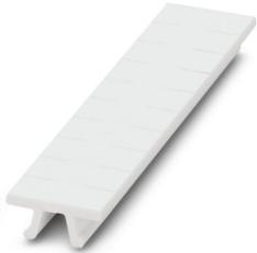
Zack marker strip, can be ordered: Strip, white, labeled according to customer specifications, mounting type: snap into tall marker groove, for terminal block width: 5.08 mm, lettering field size: 4.98 x 10.5 mm, Number of individual labels: 10
