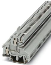
Double-level terminal block, nom. voltage: 250 V, nominal current: 12 A, number of connections: 4, number of positions: 1, connection method: Screw/plug-in connection, 1st and 2nd level connection left, cross section: 0.2 mm<sup>2</sup> - 4 mm<sup>2</sup>, mounting type: NS 35/7,5, NS 35/15, NS 32, color: gray
