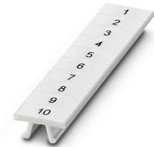
Zack marker strip, Strip, white, labeled, Printed vertically: consecutive numbers 1 ... 10, 11 ... 20, etc. up to 91 ... 100, mounting type: snapped, for terminal block width: 5.08 mm, lettering field size: 10.5 x 5.15 mm, Number of individual labels: 10
