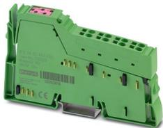
Inline, Digital output terminal, Digital outputs: 4, 24 V DC, connection technology: 3-conductor, transmission speed in the local bus: 500 kbps, degree of protection: IP20, including Inline connector
