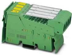
Inline, Analog output terminal, Analog outputs: 8, 0 V ... 10 V, -10 V ... 10 V, 0 V .. 5 V, -5 V ... 5 V, connection technology: 2-conductor, transmission speed in the local bus: 500 kbps, degree of protection: IP20, including Inline connectors and marking fields
