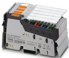
Inline, DALI master, integrated DALI power supply unit, safe electrical isolation, transmission speed in the local bus: 500 kbps, degree of protection: IP20, including Inline connectors and marking fields
