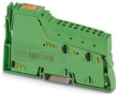
Inline, Communication terminal, interface RS-485: 1, transmission speed in the local bus: 500 kbps, degree of protection: IP20, including Inline connector
