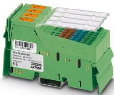
Inline, Digital input terminal, Digital inputs: 8 (S0 counter inputs), 24 V DC, connection technology: 4-conductor, transmission speed in the local bus: 500 kbps, degree of protection: IP20, including Inline connectors and marking fields
