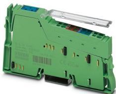
Inline, Digital input terminal, Digital inputs: 4, 24 V DC, connection technology: 3-conductor, transmission speed in the local bus: 500 kbps, degree of protection: IP20, including Inline connector and labeling field
