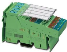
Inline, Digital input terminal, Digital inputs: 16 (NPN), 24 V DC, connection technology: 3-conductor, transmission speed in the local bus: 500 kbps, degree of protection: IP20, including Inline connectors and marking fields
