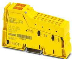
Inline, Safety module, Functional safety, Digital inputs: 4 (for 2 sensor circuits (1- or 2-channel, non-equivalent/equivalent)), Enabling current path: 1 (internal, 2-channel enabling current path), N/O contact, for safety-related shutdown of the segment voltage by means of potential routing, transmission speed in the local bus: 500 kbps, degree of protection: IP20, including Inline connectors and marking fields
