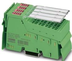
Inline, Digital output terminal, Digital outputs: 32, 24 V DC, 500 mA, connection technology: 1-conductor, transmission speed in the local bus: 500 kbps, degree of protection: IP20, including Inline connectors and marking fields
