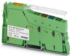
Inline, MP-Bus master terminal for connecting MP-Bus devices, transmission speed in the local bus: 500 kbps, degree of protection: IP20, including Inline connector and marking field
