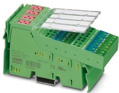
Inline, Digital output terminal, Digital outputs: 16, 24 V DC, 500 mA, connection technology: 3-conductor, transmission speed in the local bus: 500 kbps, degree of protection: IP20, including Inline connectors and marking fields
