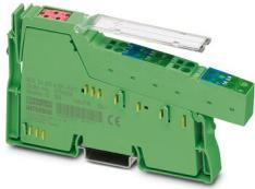
Inline, Digital output terminal, Digital outputs: 4, 24 V DC, connection technology: 3-conductor, transmission speed in the local bus: 500 kbps, degree of protection: IP20, including Inline connector and labeling field
