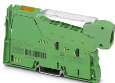
Inline, Branch terminal, for extending the Inline local bus to Inline or Fieldline Modular, transmission speed in the local bus: 500 kbps / 2 Mbps, degree of protection: IP20, including Inline connector and labeling field
