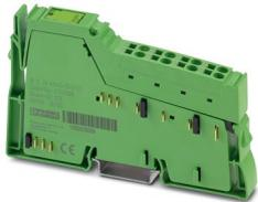
Inline, Analog input terminal, Analog inputs: 4, 0 V ... 10 V, connection technology: 2-conductor, transmission speed in the local bus: 500 kbps, degree of protection: IP20, including Inline connector
