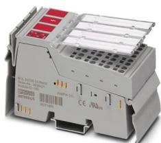
Inline, Relay terminal, Relay outputs: 4 (floating), Changeover contact, 24 V DC, 230 V AC, for switching ohmic loads, transmission speed in the local bus: 500 kbps, degree of protection: IP20, including Inline connectors and marking fields
