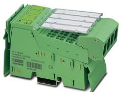
Inline, Analog input terminal, Analog inputs: 8, 0 mA ... 20 mA, 4 mA ... 20 mA, -20 mA ... 20 mA, 0 mA ... 40 mA, -40 mA ... 40 mA, connection technology: 2-, 3-conductor, transmission speed in the local bus: 500 kbps, integrated sensor supply, degree of protection: IP20, including Inline connectors and marking fields
