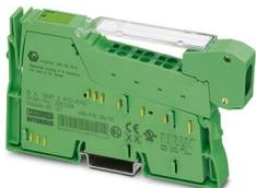
Inline, Temperature measurement terminal, Analog RTD inputs: 2, connection technology: 2-, 3-, 4-conductor, transmission speed in the local bus: 500 kbps, degree of protection: IP20, including Inline connector and labeling field
