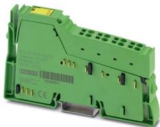
Inline, Analog output terminal, Analog outputs: 4, 4 mA ... 20 mA, connection technology: 2-conductor, transmission speed in the local bus: 500 kbps, degree of protection: IP20, including Inline connector
