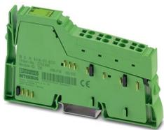
Inline, Analog input terminal, Analog inputs: 4, 4 mA ... 20 mA, connection technology: 2-conductor, transmission speed in the local bus: 500 kbps, degree of protection: IP20, including Inline connector
