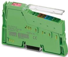
Inline, Digital output terminal, Digital outputs: 2, 24 V DC, connection technology: 4-conductor, transmission speed in the local bus: 500 kbps, degree of protection: IP20, including Inline connector and labeling field
