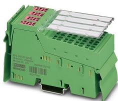
Inline, Digital output terminal, Digital outputs: 32 (NPN), 24 V DC, connection technology: 1-conductor, transmission speed in the local bus: 500 kbps, degree of protection: IP20, including Inline connectors and marking fields
