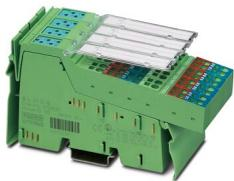
Inline, Digital input terminal, Digital inputs: 16, 24 V DC, connection technology: 3-conductor, transmission speed in the local bus: 500 kbps, degree of protection: IP20, including Inline connectors and marking fields, connectors numbered individually
