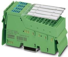
Inline, Digital input terminal, Digital inputs: 32, 24 V DC, connection technology: 1-conductor, transmission speed in the local bus: 500 kbps, degree of protection: IP20, including Inline connectors and marking fields
