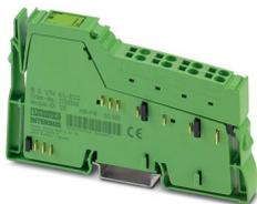
Inline ECO, Temperature measurement terminal, Analog UTH inputs: 4 (Type L), connection technology: 2-conductor, transmission speed in the local bus: 500 kbps, degree of protection: IP20, including Inline connector
