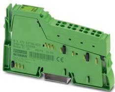
Inline, Temperature measurement terminal, Analog RTD inputs: 4 (Pt 100), connection technology: 2-conductor, transmission speed in the local bus: 500 kbps, degree of protection: IP20, including Inline connector
