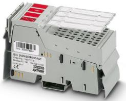
Inline, Relay terminal, Relay outputs: 4 (floating), N/O contact, 24 V DC, 230 V AC, high inrush current, transmission speed in the local bus: 500 kbps, degree of protection: IP20, including Inline connectors and marking fields
