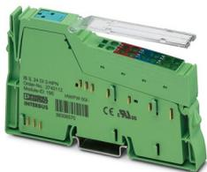
Inline, Digital input terminal, Digital inputs: 2 (NPN), 24 V DC, connection technology: 4-conductor, transmission speed in the local bus: 500 kbps, degree of protection: IP20, including Inline connector and labeling field
