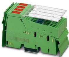
Inline, Digital output terminal, Digital outputs: 16, 24 V DC, connection technology: 3-conductor, transmission speed in the local bus: 500 kbps, degree of protection: IP20, including Inline connectors and marking fields
