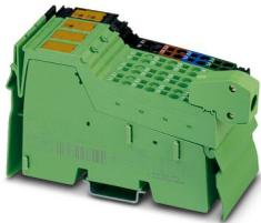
Inline, Coupler terminal, for extending the Inline local bus, transmission speed in the local bus: 500 kbps / 2 Mbps, degree of protection: IP20, including Inline connectors and marking fields
