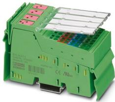
Inline, Digital output terminal, Digital outputs: 8, 24 V DC, connection technology: 4-conductor, transmission speed in the local bus: 500 kbps, degree of protection: IP20, including Inline connectors and marking fields
