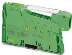
Inline, Analog input terminal, Analog inputs: 2, 0 V ... 10 V, -10 V ... 10 V, 0 mA ... 20 mA, 4 mA ... 20 mA, -20 mA ... 20 mA, connection technology: 2-conductor, transmission speed in the local bus: 500 kbps, degree of protection: IP20, including Inline connector and labeling field
