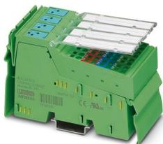
Inline, Digital input terminal, Digital inputs: 8, 24 V DC, connection technology: 4-conductor, transmission speed in the local bus: 500 kbps, degree of protection: IP20, including Inline connectors and marking fields
