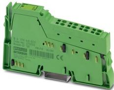
Inline, Temperature measurement terminal, Analog UTH inputs: 4 (Type K), connection technology: 2-conductor, transmission speed in the local bus: 500 kbps, degree of protection: IP20, including Inline connector
