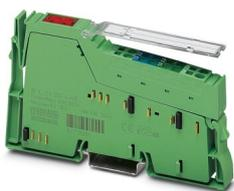
Inline, Digital output terminal, Digital outputs: 4, 24 V DC, connection technology: 3-conductor, transmission speed in the local bus: 500 kbps, degree of protection: IP20, including Inline connector and labeling field
