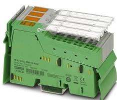
Inline, DALI master, Multi-master-capable, integrated DALI power supply unit, transmission speed in the local bus: 500 kbps, degree of protection: IP20, including Inline connectors and marking fields
