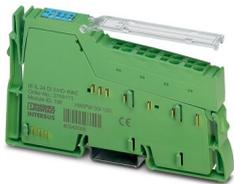
Inline, Digital input terminal, Digital inputs: 8, 24 V DC, connection technology: 1-conductor, transmission speed in the local bus: 500 kbps, degree of protection: IP20, including Inline connector and labeling field
