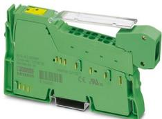
Inline, Analog output terminal, Analog outputs: 2, 0 V ... 10 V, -10 V ... 10 V, connection technology: 2-conductor, transmission speed in the local bus: 500 kbps, degree of protection: IP20, including Inline connector and labeling field
