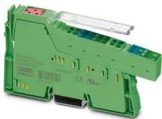
Inline, Digital output terminal, Digital outputs: 4, 24 V DC, 500 mA, connection technology: 3-conductor, transmission speed in the local bus: 500 kbps, degree of protection: IP20, including Inline connector and labeling field
