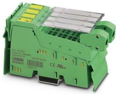
Inline, Analog output terminal, Analog outputs: 2, 0 V ... 10 V, 0 mA ... 20 mA, 4 mA ... 20 mA, connection technology: 2-conductor, transmission speed in the local bus: 500 kbps, degree of protection: IP20, including Inline connectors and marking fields
