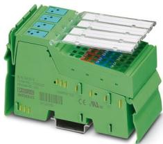
Inline, Digital input terminal, Digital inputs: 8, 24 V DC, connection technology: 4-conductor, transmission speed in the local bus: 500 kbps, degree of protection: IP20, including Inline connectors and marking fields
