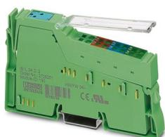
Inline, Digital input terminal, Digital inputs: 2, 24 V DC, connection technology: 4-conductor, transmission speed in the local bus: 500 kbps, degree of protection: IP20, including Inline connector and labeling field
