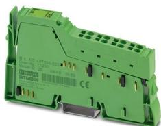
Inline, Temperature measurement terminal, Analog RTD inputs: 4 (Pt 1000), connection technology: 2-conductor, transmission speed in the local bus: 500 kbps, degree of protection: IP20, including Inline connector
