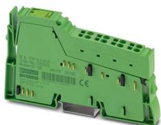
Inline, Temperature measurement terminal, Analog UTH inputs: 4 (Type J), connection technology: 2-conductor, transmission speed in the local bus: 500 kbps, degree of protection: IP20, including Inline connector
