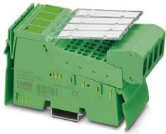
Inline, Analog input terminal, Analog inputs: 8, 0 V ... 5 V, -5 V ... 5 V, 0 V ... 10 V, -10 V ... 10 V, 0 V ... 25 V, -25 V ... 25 V, 0 V ... 50 V, 0 mA ... 20 mA, 4 mA ... 20 mA, -20 mA ... 20 mA, 0 mA ... 40 mA, -40 mA ... 40 mA, connection technology: 2-conductor, transmission speed in the local bus: 500 kbps, degree of protection: IP20, including Inline connectors and marking fields
