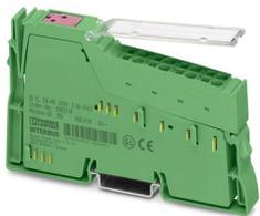
Inline, Relay terminal, Relay outputs: 2 (floating), Changeover contact, 24 V AC, 48 V DC, for switching ohmic loads, transmission speed in the local bus: 500 kbps, degree of protection: IP20, including Inline connector and labeling field
