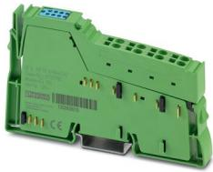
Inline, Digital input terminal, Digital inputs: 8, 24 V DC, connection technology: 1-conductor, transmission speed in the local bus: 500 kbps, degree of protection: IP20, including Inline connector
