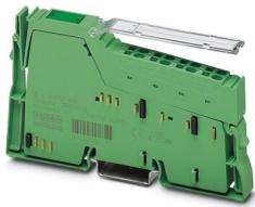
Inline, Analog input terminal, Analog inputs: 2, 0 V ... 10 V, -10 V ... 10 V, 0 mA ... 20 mA, 4 mA ... 20 mA, -20 mA ... 20 mA, connection technology: 2-conductor, transmission speed in the local bus: 500 kbps, degree of protection: IP20, including Inline connector and labeling field
