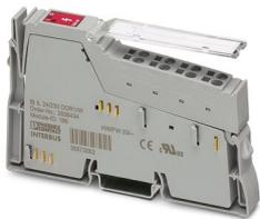
Inline, Relay terminal, Relay output: 1 (floating contacts), 24 V DC, 230 V AC, for switching inductive and capacitive loads, transmission speed in the local bus: 500 kbps, degree of protection: IP20, including Inline connector and labeling field
