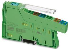
Inline, Digital input terminal, Digital inputs: 4, 24 V DC, connection technology: 3-conductor, transmission speed in the local bus: 500 kbps, degree of protection: IP20, including Inline connector and labeling field
