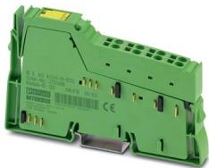
Inline, Analog output terminal, Analog outputs: 4, 0 V ... 10 V, connection technology: 2-conductor, transmission speed in the local bus: 500 kbps, degree of protection: IP20, including Inline connector
