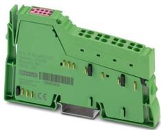
Inline, Digital output terminal, Digital outputs: 8, 24 V DC, connection technology: 1-conductor, transmission speed in the local bus: 500 kbps, degree of protection: IP20, including Inline connector
