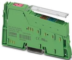
Inline, Digital output terminal, Digital outputs: 2 (NPN), 24 V DC, connection technology: 4-conductor, transmission speed in the local bus: 500 kbps, degree of protection: IP20, including Inline connector and labeling field
