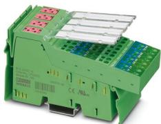
Inline, Digital output terminal, Digital outputs: 16, 24 V DC, 500 mA, connection technology: 3-conductor, transmission speed in the local bus: 500 kbps, degree of protection: IP20, including Inline connectors and marking fields, connectors numbered individually
