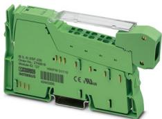
Inline, Analog input terminal, Analog inputs: 2, 0 V ... 10 V, -10 V ... 10 V, 0 mA ... 20 mA, 4 mA ... 20 mA, -20 mA ... 20 mA, connection technology: 2-conductor, transmission speed in the local bus: 500 kbps, 3 dB base frequency at 230 Hz, degree of protection: IP20, including Inline connector and labeling field
