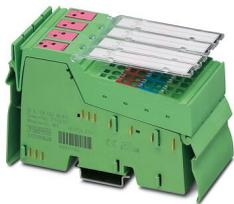
Inline, Digital output terminal, Digital outputs: 8, 24 V DC, connection technology: 4-conductor, transmission speed in the local bus: 500 kbps, degree of protection: IP20, including Inline connectors and marking fields
