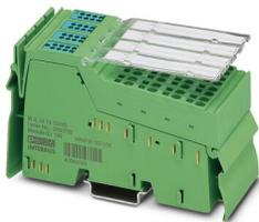
Inline, Digital input terminal, Digital inputs: 32 (NPN), 24 V DC, connection technology: 1-conductor, transmission speed in the local bus: 500 kbps, degree of protection: IP20, including Inline connectors and marking fields
