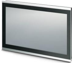
Touch panel with 47.0 cm / 18.5" TFT-display (projective-capacitive (PCAP)), 1366 x 768 pixel(s) (WXGA), 65536 colors, Arm<sup>®</sup> Cortex<sup>®</sup>-A8, 1000 MHz, 2x USB host 2.0, 1 x Ethernet (10/100 Mbps), RJ45, Windows<sup>®</sup> Embedded Compact 7 and user software: Visu+. (bus system: without)
