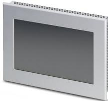
Touch panel with 17.8 cm/7" TFT-display (analog resistive (polyester)), 800 x 480 pixel(s) (WVGA), 262144 colors, Arm® Cortex®-A8, 800 MHz, 2x USB host 2.0, 1 x Ethernet (10/100 Mbps), RJ45, Windows® Embedded Compact 7 and user software: Visu+ / AX OPC Server. (bus system: without)
