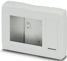
Display housing, 5.7", light gray, consisting of two half shells with screws, window on the left. Front 1.1 mm recessed, keypad area on the right recessed for wall installation
