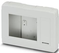
Display housing, 5.7", light gray, consisting of two half shells, four front plates with screws and battery pack contacts, window on the left. Front 1.1 mm recessed, keypad area on the right, recessed for battery pack
