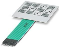
Membrane keypad, self-adhesive, silver conduction technology, 12 keys, embossed, 3 colors, connecting cable: 100.5 mm, with crimp female connector, pitch: 2.54 mm, operating temperature: -20°C ... 70°C
