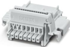
DIN rail connector, color: light grey, nominal current: 6 A (parallel contacts), rated voltage (III/2): 32 V, number of positions: 8, pitch: 2.54 mm, mounting: DIN rail mounting, locking: without, mounting: without, type of packaging: packed in cardboard, Item with gold-plated contacts, bus connectors for connecting with electronics housings, 8 parallel contacts
