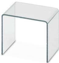
Press-drawn section housings, Latching, Cover, color: transparent, width: 73 mm, profile length (configurable): 3 cm ... 100 cm, height: 63.2 mm, Note: max. length of the cover = PCB length - 19 mm
