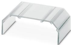
Press-drawn section housings, Latching, Cover, color: transparent, width: 92 mm, profile length (configurable): 3 cm ... 100 cm, height: 34 mm, Note: max. length of the cover = PCB length - 19 mm
