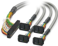
Round cable set; controller: Allen-Bradley SLC 500 (IB 32); connection 1: IDC/FLK socket strip (1x 40-position); connection 2: IDC/FLK socket strip (4x 14-position); cable length: 2 m
