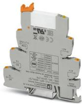
PLC-INTERFACE, consisting of PLC-BPT.../21 basic terminal block with Push-in connection and plug-in miniature relay with multi-layer gold contact, for mounting on DIN rail NS 35/7,5, 1 changeover contact, input voltage 60 V DC
