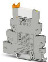
PLC-INTERFACE, consisting of PLC-BSC.../21 basic terminal block with screw connection and plug-in miniature relay with multi-layer gold contact, for mounting on DIN rail NS 35/7,5, 1 changeover contact, input voltage 60 V DC
