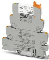
PLC-INTERFACE for input functions, consisting of PLC-BPT.../SEN basic terminal block with push-in connection and plug-in miniature relay with multi-layer gold contact, for mounting on DIN rail NS 35/7,5, 1 N/O contact, input voltage 230 V AC/220 V DC
