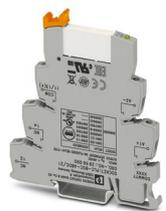
PLC-INTERFACE, consisting of PLC-BSC.../21 basic terminal block with screw connection and plug-in miniature relay with multi-layer gold contact, for mounting on DIN rail NS 35/7,5, 1 changeover contact, input voltage 48 V DC
