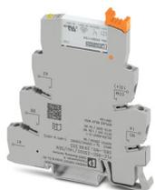
PLC-INTERFACE for input functions, consisting of PLC-BSC.../SEN basic terminal block with screw connection and plug-in miniature relay with multi-layer gold contact, for mounting on DIN rail NS 35/7,5, 1 N/O contact, input voltage 230 V AC/220 V DC
