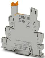
6.2 mm PLC basic terminal block with protection against interference currents/voltages on the control side, with screw connection, without relay or solid-state relay, for mounting on DIN rail NS 35/7,5, with integrated RCZ filter, 1 changeover contact, input voltage 120 V AC
