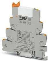
PLC-INTERFACE, consisting of PLC-BPT.../21 basic terminal block with Push-in connection and plug-in miniature relay with multi-layer gold contact, for mounting on DIN rail NS 35/7,5, 1 changeover contact, input voltage 48 V DC
