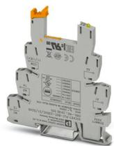
6.2 mm PLC basic terminal block with protection against interference currents/voltages on the control side, with screw connection, without relay or solid-state relay, for mounting on DIN rail NS 35/7,5, with integrated RCZ filter, 1 changeover contact, input voltage 230 V AC
