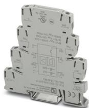
PLC-INTERFACE for NAMUR applications, consisting of PLC-BSC.../21 basic terminal block with screw connection and integrated circuit, for mounting on NS 35/7,5 DIN rail, positive switching output, 24 V DC supply voltage
