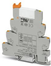
PLC-INTERFACE, consisting of PLC-BPT.../21 basic terminal block with Push-in connection and plug-in miniature relay with multi-layer gold contact, for mounting on DIN rail NS 35/7,5, 1 changeover contact, input voltage 12 V DC
