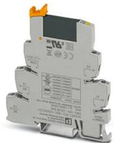
PLC-INTERFACE, consisting of PLC-BSC.../21 basic terminal block with screw connection and plug-in miniature solid-state relay, for mounting on DIN rail NS 35/7,5, 1 N/O contact, input: 230 V AC/220 V DC, output: 3 - 48 V DC/100 mA
