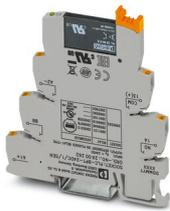
PLC-INTERFACE for input functions, consisting of PLC-BPT.../SEN basic terminal block with push-in connection and plug-in miniature solid-state relay, for mounting on DIN rail NS 35/7,5, 1 N/O contact, input: 24 V DC, output: 3 - 48 V DC/100 mA
