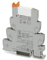
PLC-INTERFACE, consisting of PLC-BSC.../21 basic terminal block with screw connection and plug-in miniature relay with multi-layer gold contact, for mounting on DIN rail NS 35/7,5, 1 changeover contact, input voltage 12 V DC
