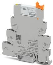
PLC-INTERFACE for input functions, consisting of PLC-BSC.../SEN basic terminal block with screw connection and plug-in miniature relay with multi-layer gold contact, for mounting on DIN rail NS 35/7,5, 1 N/O contact, input voltage 24 V DC
