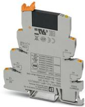
PLC-INTERFACE, consisting of PLC-BPT.../21 basic terminal block with push-in connection and plug-in miniature solid-state relay, for mounting on DIN rail NS 35/7,5, 1 N/O contact, input: 230 V AC/220 V DC, output: 3 - 48 V DC/100 mA
