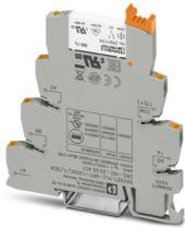
PLC-INTERFACE for input functions, consisting of PLC-BPT.../SEN basic terminal block with push-in connection and plug-in miniature relay with multi-layer gold contact, for mounting on DIN rail NS 35/7,5, 1 N/O contact, input voltage 120 V AC/110 V DC
