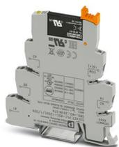
PLC-INTERFACE for input functions, consisting of PLC-BSC.../SEN basic terminal block with screw connection and plug-in miniature solid-state relay, for mounting on DIN rail NS 35/7,5, 1 N/O contact, input: 120 V AC/110 V DC, output: 3 - 48 V DC/100 mA
