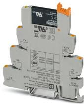
PLC-INTERFACE for input functions, consisting of PLC-BPT.../SEN basic terminal block with push-in connection and plug-in miniature solid-state relay, for mounting on DIN rail NS 35/7,5, 1 N/O contact, input: 230 V AC/220 V DC, output: 3 - 48 V DC/100 mA
