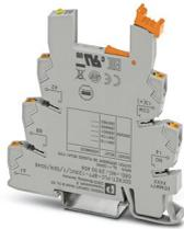
6.2 mm PLC basic terminal block with interference current and interference voltage protection on the control side, with push-in connection, without relay or solid-state relay, with sensor supply voltage distribution (BB), 1 N/O contact, input voltage 120 V AC
