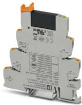
PLC-INTERFACE, consisting of PLC-BPT.../21 basic terminal block with push-in connection and plug-in miniature solid-state relay, for mounting on DIN rail NS 35/7,5, 1 N/O contact, input: 120 V AC/110 V DC, output: 3 - 48 V DC/100 mA
