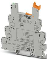
6.2 mm PLC basic terminal block with interference current and interference voltage protection on the control side, with screw connection, without relay or solid-state relay, with sensor supply voltage distribution (BB), 1 N/O contact, input voltage 230 V AC
