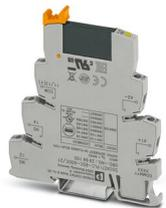
PLC-INTERFACE, consisting of PLC-BSC.../21 basic terminal block with screw connection and plug-in miniature solid-state relay, for mounting on DIN rail NS 35/7,5, 1 N/O contact, input: 60 V DC, output: 3 - 48 V DC/100 mA
