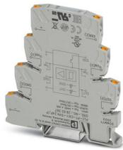
PLC-INTERFACE for NAMUR applications, consisting of PLC-BPT.../21 basic terminal block with Push-in connection and integrated circuit, for mounting on NS 35/7,5 DIN rail, positive switching output, 24 V DC supply voltage
