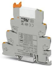
PLC-INTERFACE, consisting of PLC-BPT.../21 basic terminal block with Push-in connection and plug-in miniature relay with multi-layer gold contact, for mounting on DIN rail NS 35/7,5, 1 changeover contact, input voltage 120 V AC/110 V DC
