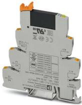
PLC-INTERFACE, consisting of PLC-BPT.../21 basic terminal block with push-in connection and plug-in miniature solid-state relay, for mounting on DIN rail NS 35/7,5, 1 N/O contact, input: 24 V DC, output: 3 - 48 V DC/100 mA
