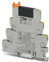
PLC-INTERFACE, consisting of PLC-BPT.../21 basic terminal block with push-in connection and plug-in miniature solid-state relay, for mounting on DIN rail NS 35/7,5, 1 N/O contact, input: 60 V DC, output: 3 - 48 V DC/100 mA
