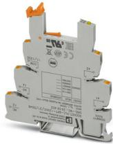
6.2 mm PLC basic terminal block against interference currents/voltages on the control side with Push-in connection, without relay or solid-state relay, for mounting on DIN rail NS 35/7,5, with integrated RCZ filter, 1 changeover contact, input voltage 120 V AC
