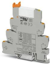
PLC-INTERFACE, consisting of PLC-BPT.../21 basic terminal block with Push-in connection and plug-in miniature relay with multi-layer gold contact, for mounting on DIN rail NS 35/7,5, 1 changeover contact, input voltage 230 V AC/220 V DC
