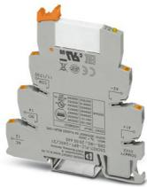
PLC-INTERFACE, consisting of PLC-BPT.../21 basic terminal block with Push-in connection and plug-in miniature relay with multi-layer gold contact, for mounting on DIN rail NS 35/7,5, 1 changeover contact, input voltage 24 V DC
