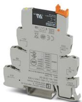
PLC-INTERFACE for input functions, consisting of PLC-BSC.../SEN basic terminal block with screw connection and plug-in miniature solid-state relay, for mounting on DIN rail NS 35/7,5, 1 N/O contact, input: 24 V DC, output: 3 - 48 V DC/100 mA
