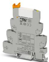
PLC-INTERFACE, consisting of PLC-BSC.../21 basic terminal block with screw connection and plug-in miniature relay with multi-layer gold contact, for mounting on DIN rail NS 35/7,5, 1 changeover contact, input voltage 24 V AC/DC
