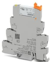
PLC-INTERFACE for input functions, consisting of PLC-BSC.../SEN basic terminal block with screw connection and plug-in miniature relay with multi-layer gold contact, for mounting on DIN rail NS 35/7,5, 1 N/O contact, input voltage 120 V AC/110 V DC
