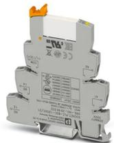
PLC-INTERFACE, consisting of PLC-BSC.../21 basic terminal block with screw connection and plug-in miniature relay with multi-layer gold contact, for mounting on DIN rail NS 35/7,5, 1 changeover contact, input voltage 120 V AC/110 V DC
