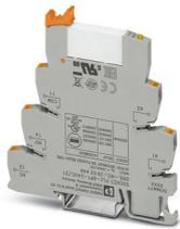
PLC-INTERFACE, consisting of PLC-BPT.../21 basic terminal block with Push-in connection and plug-in miniature relay with multi-layer gold contact, for mounting on DIN rail NS 35/7,5, 1 changeover contact, input voltage 24 V AC/DC
