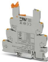
6.2 mm PLC basic terminal block against interference currents/voltages on the control side with Push-in connection, without relay or solid-state relay, for mounting on DIN rail NS 35/7,5, with integrated RCZ filter, 1 changeover contact, input voltage 230 V AC
