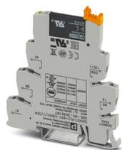
PLC-INTERFACE for input functions, consisting of PLC-BSC.../SEN basic terminal block with screw connection and plug-in miniature solid-state relay, for mounting on DIN rail NS 35/7,5, 1 N/O contact, input: 230 V AC/220 V DC, output: 3 - 48 V DC/100 mA
