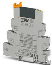
PLC-INTERFACE, consisting of PLC-BSC.../21 basic terminal block with screw connection and plug-in miniature solid-state relay, for mounting on DIN rail NS 35/7,5, 1 N/O contact, input: 48 V DC, output: 3 - 48 V DC/100 mA
