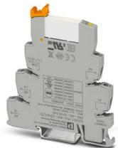
PLC-INTERFACE, consisting of PLC-BSC.../21 basic terminal block with screw connection and plug-in miniature relay with multi-layer gold contact, for mounting on DIN rail NS 35/7,5, 1 changeover contact, input voltage 230 V AC/220 V DC
