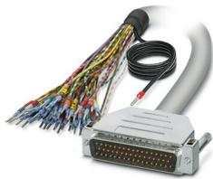
Assembled shielded round cable; connection 1: Single wires (50-position) (The wires are marked and fitted with ferrules. The braided shield is routed to a separate cable end.); connection 2: D-SUB pin strip (1x 50-position); cable length: 3 m
