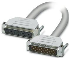
Assembled shielded round cable; connection 1: D-SUB socket strip (1x 50-position); connection 2: D-SUB pin strip (1x 50-position); cable length: 1 m
