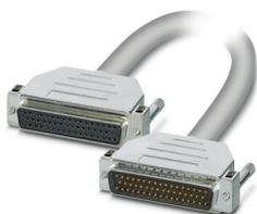
Assembled shielded round cable; connection 1: D-SUB socket strip (1x 50-position); connection 2: D-SUB pin strip (1x 50-position); cable length: 0.5 m
