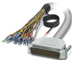
Assembled shielded round cable; connection 1: Single wires (50-position) (The wires are marked and fitted with ferrules. The braided shield is routed to a separate cable end.); connection 2: D-SUB pin strip (1x 50-position); cable length: variable
