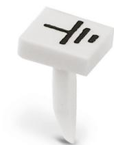
Marker pin, Stud, white, labeled, horizontal: Symbols +,-,/~,ERD,SERD, L1, L2, L3 PE, PEN (up to 3 characters), mounting type: plug in, for terminal block width: 4.2 mm, lettering field size: 4 x 4 mm, Number of individual labels: 1
