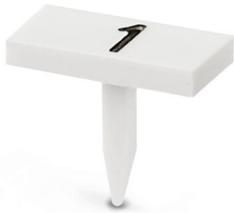
Zack marker strip, Stud, white, labeled, mounting type: plug in, for terminal block width: 7.5 mm, lettering field size: 4 x 7.5 mm, Number of individual labels: 1
