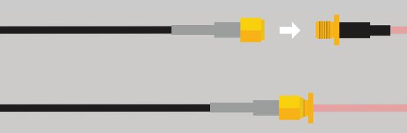
If you need to water proof a SMA connection, we highly recommend using a product like Coax-Seal to safely cover and prevent any water damage that may occur.
