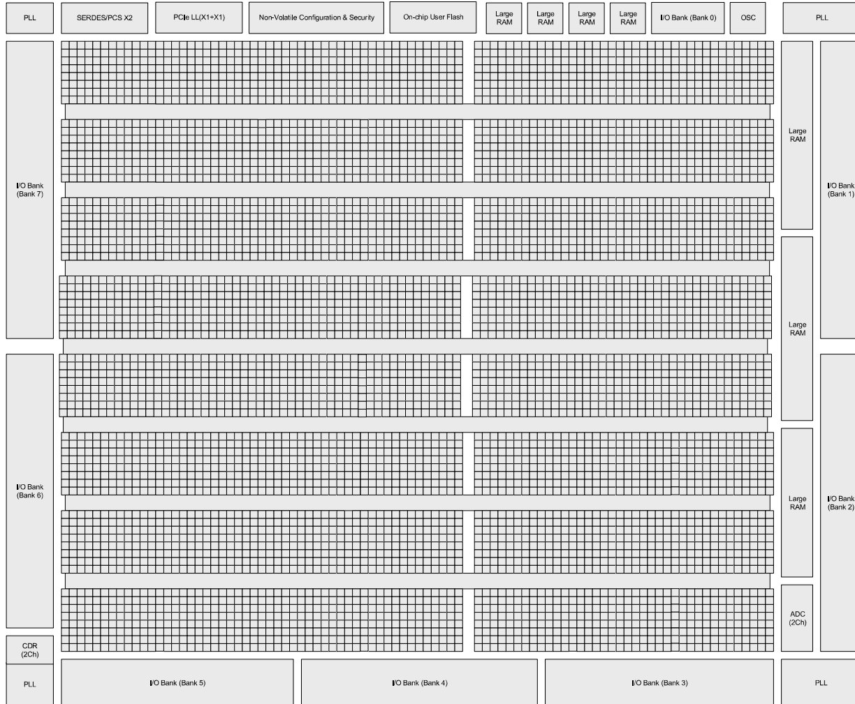
Figure 2.3. Simplified Block Diagram, MachXO5-NX-100T Device (Top Level)
