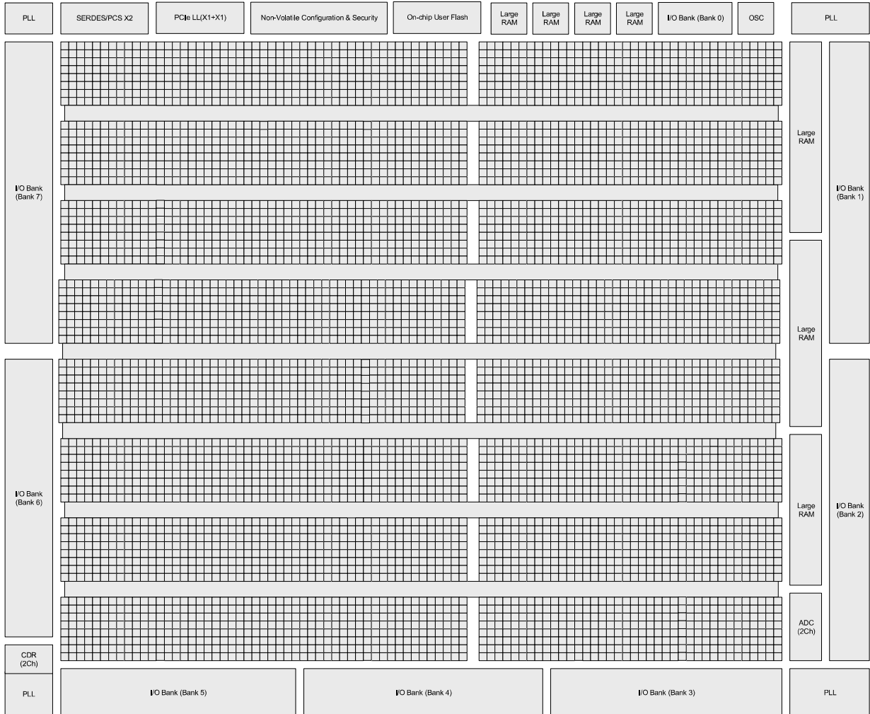
Figure 2.2. Simplified Block Diagram, MachXO5-NX-55T Device (Top Level)
