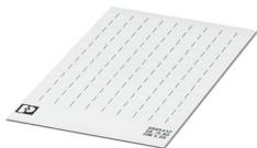
Marker card, white, unlabeled, can be labeled with: Marker pen: without print, mounting type: adhesive, for terminal block width: 5.08 mm, lettering field size: 5.08 x 3.8 mm, Number of individual labels: 120
