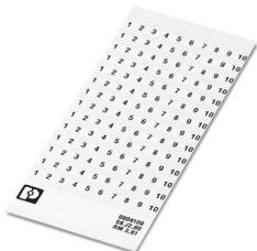
Marker card, white, labeled, horizontal: consecutive numbers 1 ... 10, 11 ... 20, etc. up to 91 ... (99)100, mounting type: adhesive, for terminal block width: 3.81 mm, lettering field size: 3.81 x 2.8 mm
