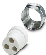
Multiple screw connection Pg21, made of metal, consisting of rubber seal with several holes (3 x 7 mm) and a pressure screw, for cable screw connection thread VC-M-KV-PG21...
