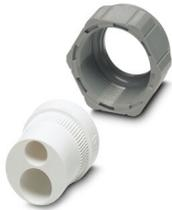
Half screw connection Pg21, made of plastic, consisting of rubber seal with several holes (1 x 8.5 mm/1 x 12 mm) and a pressure screw, for cable screw connection thread VC-M-KV-PG21.....
