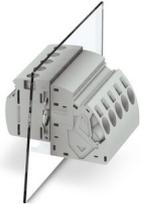
Panel feed-through terminal block, connection method: Push-in spring connection, Screw connection with tension sleeve, number of positions: 1, load current: 76 A, cross section: 1.5 mm<sup>2</sup> - 16 mm<sup>2</sup>, connection direction of the conductor to plug-in direction: 45 °, width: 12 mm
