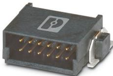
SMD male connector, nominal current: 1.4 A, Test voltage: 500 V AC, number of positions: 40, pitch: 1.27 mm, color: black, contact surface: Gold, contact connection type: Pin, mounting: SMD soldering
