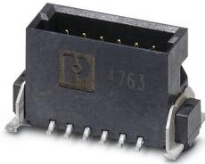
SMD male connector, nominal current: 1.4 A, Test voltage: 500 V AC, number of positions: 40, pitch: 1.27 mm, color: black, contact surface: Gold, contact connection type: Pin, mounting: SMD soldering
