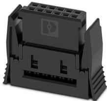
IDC female connector, nominal current: 1.2 A, Test voltage: 500 V AC, number of positions: 40, pitch: 1.27 mm, number of rows: 2, color: black, contact surface: Gold, contact connection type: Socket, For preassembled samples, see the "Accessories" tab.
