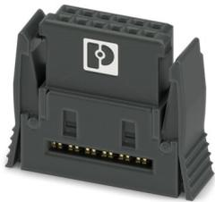
IDC female connector, nominal current: 1.2 A, Test voltage: 500 V AC, number of positions: 12, pitch: 1.27 mm, number of rows: 2, connection method: IDC connection, color: black, contact surface: Gold, contact connection type: Socket, For preassembled samples, see the "Accessories" tab.
