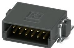
SMD male connector, nominal current: 1.4 A, Test voltage: 500 V AC, number of positions: 12, pitch: 1.27 mm, color: black, contact surface: Gold, contact connection type: Pin, mounting: SMD soldering
