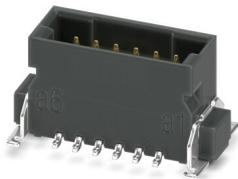
SMD male connector, nominal current: 1.4 A, Test voltage: 500 V AC, number of positions: 12, pitch: 1.27 mm, color: black, contact surface: Gold, contact connection type: Pin, mounting: SMD soldering
