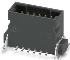
SMD male connector, nominal current: 1.4 A, Test voltage: 500 V AC, number of positions: 12, pitch: 1.27 mm, color: black, contact surface: Gold, contact connection type: Pin, mounting: SMD soldering
