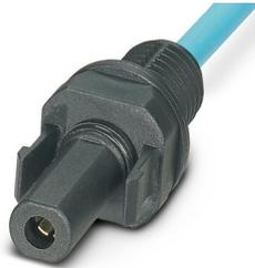
Panel feed-through, Range of articles: Sunclix, Device connector front mounting, housing material: PPE, color: black, min. conductor cross section: 4 mm<sup>2</sup>, Connection method: Crimp, Contact connection type: Socket, cable length: 170
