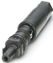
Photovoltaic connector, Range of articles: Sunclix, Connector, housing material: PPE, color: black, number of positions: 1, min. conductor cross section: 2.5 mm<sup>2</sup>, max. conductor cross section: 6 mm<sup>2</sup>, rated current: 27 A, Connection method: Spring-cage, Contact connection type: Socket
