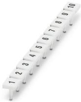
Marker pin Zack strip, Strip, white, labeled, printed horizontally: consecutive numbers 1 ... 10, 11 ... 20, etc. up to 491 ... 500, mounting type: plug in, for terminal block width: 5 mm, lettering field size: 4 x 4 mm, Number of individual labels: 10
