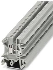
Feed-through terminal block, nom. voltage: 250 V, nominal current: 12 A, number of connections: 3, number of positions: 1, connection method: Screw/plug-in connection, 2nd level connection left, cross section: 0.2 mm<sup>2</sup> - 4 mm<sup>2</sup>, mounting type: NS 32, NS 35/15, NS 35/7,5, color: gray
