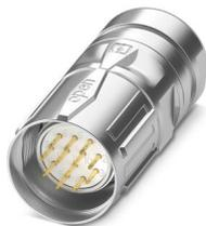
M23, Cable connector, series: CA, straight, shielded: yes, SPEEDCON, No. of pos.: 16, Direction of rotation: Standard, contact connection type: Pin, Solder connection, cable diameter range: 6 mm ... 10 mm, coding: N, Alternative product in accordance with RoHS II without Exemption 6c (Pb <0.1%) item no.: 1243627
