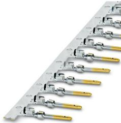
Crimp contact, Pin, rolled, Taped articles, number of pieces per reel: 500, contact diameter: 1 mm, crimp range: 0.22 mm<sup>2</sup> ... 0.56 mm<sup>2</sup>, Item is lead-free in accordance with RoHS II without Exemption 6c (Pb <0.1%)
