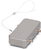
Protective cover B16, for double locking latch, protective cover material: Al, height: 16 mm, seal: no, with lanyard
