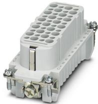
Contact insert, number of positions: 40+PE, size: B16, number of connections per position: 1, Socket, Crimp connection, 250 V, 10 A, 0.14 mm<sup>2</sup> ... 2.5 mm<sup>2</sup>, application: Signal
