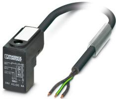
Sensor/actuator cable, 3-position halogen-free, free cable end, on Valve connector CI (9.4 mm), with 1 LED, connected with Z diode, cable length: 5 m
