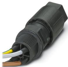
Panel feed-through, QUICKON connection, number of positions: 3+PE, 1 mm<sup>2</sup> ... 2.5 mm<sup>2</sup>, 690 V, 20 A, black, with QUICKON nut, external cable diameter: 9 mm ... 14 mm, assembly thread: M25, IDC connection (welded-on), 2.5 mm<sup>2</sup>, wires cut flat at the end, cable length: 1 m
