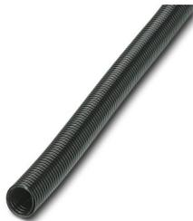
Protective hose, material: PA 6, UV-resistant: yes, flexible, degree of protection: IP68, color: black, flammability rating in acc. with UL 94: V0, inner diameter: 10 mm, Total length: 50 m
