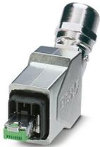
Push-pull connector (version 14), die-cast zinc, with RJ45 connector insert, 8-pos., with IDC fast connection technology, for 1 and 7-wire cores, 26 ... 24 AWG, for cable diameter of 5.5 mm ... 10 mm
