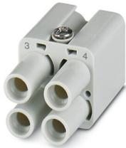
Contact insert, number of positions: 4, size: D7, number of connections per position: 1, Socket, Crimp connection, 830 V, 40 A, 1.5 mm<sup>2</sup> ... 6 mm<sup>2</sup>, application: Power, Only suitable for plastic housings
