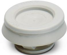
Membrane screw connection, material for screw connection: Polypropylene, external cable diameter 4 mm ... 10 mm, shielding: no, connecting thread: M16, color: light grey
