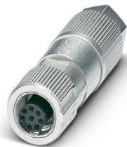
Connector, Universal, 8-position, halogen-free, shielded, Socket straight M12, A, Insulation displacement connection, knurl material: Zinc die-cast, nickel-plated, external cable diameter 5 mm ... 9.7 mm
