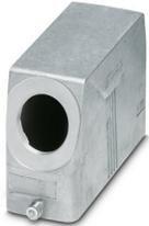
Sleeve housing B24, for single locking latch, material: Die-cast aluminum, salt water resistant, cable outlets: 1, lateral, 1x M40, height: 76 mm, cable gland: none, Standard
