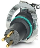
Contact carrier, 3-position, Pin, straight, M8, coding: A, PCB mounting, SMD reflow, Alternative product in accordance with RoHS II without Exemption 6c (Pb <0.1%) item no.: 1308281
