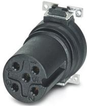
Contact carrier, 4-position, Socket, straight, M12, coding: A, PCB mounting, SMD reflow, Alternative product in accordance with RoHS II without Exemption 6c (Pb <0.1%) item no.: 1238915
